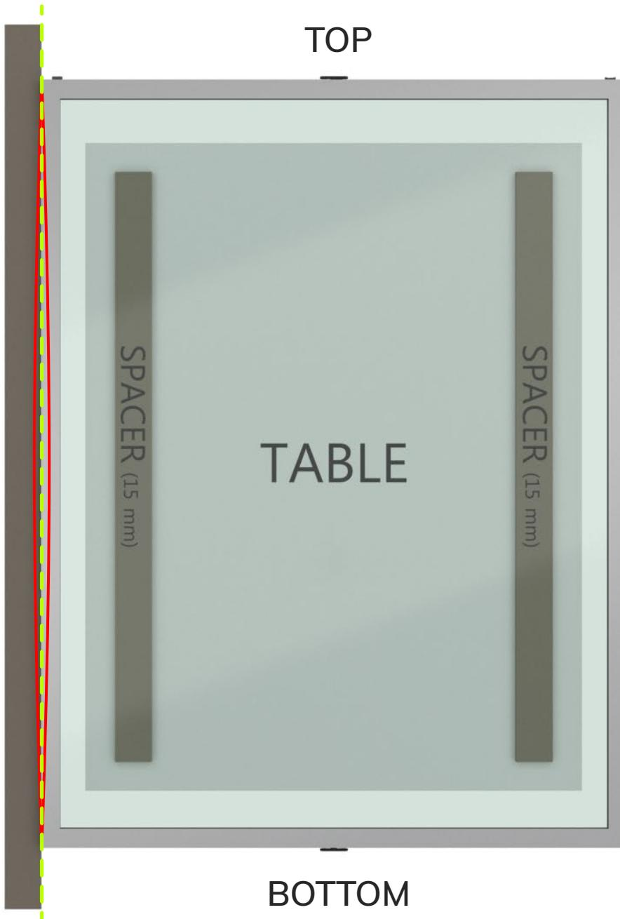
Make sure the starting profile is 100% straight! If not, use a rubber hammer to straighten profile.
