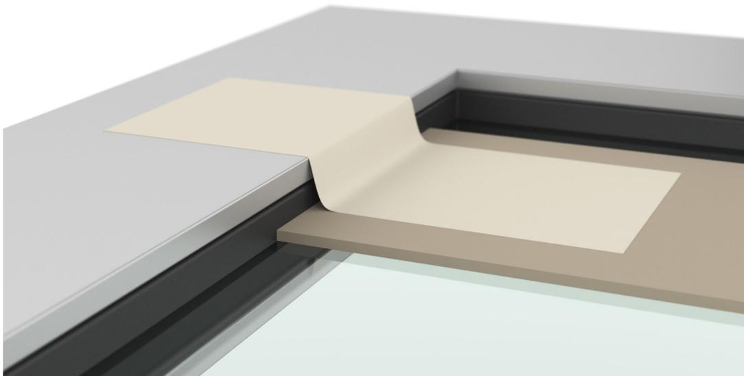
Use masking tape to keep the guide in place.
