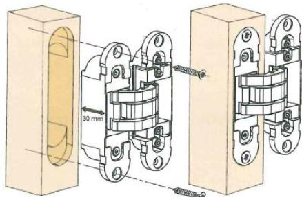
Insert the part of the hinge marked as 'door' (depth 30 mm) in the milling of the door, then fix the hinge by screwing with suitable wood screws.
